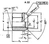
Screw thread countersunk down to thread diameter.
