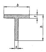
Designation of a hot rolled T-bar, sharp-edged (TPS), of depth  $h=30\,\mathrm{mm}$  produced from a steel with code number St 37-2 or material number 1.0037 according to DIN 17 100:
