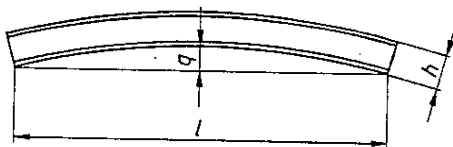
Figure 4: Deviation from straightness of vertical web
