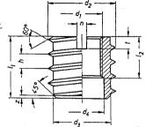
Designation of a screwed insert with thread  $d_4$  = M 6 and length  $l_4$  = 15 mm, in St: Screwed insert M 6 x 15 DIN 7965 - St
