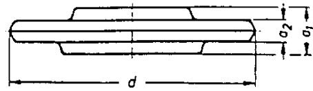
Figure 4. Exceptional case for thin discs or flanges
