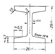
Designation of a rolled I-steel of 29 mm height and 26 mm width:  $I\text{-steel }29 \times 26 \text{ DIN }6634$
