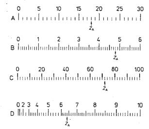
In the case of scale pattern A the scale divisions are counted continuously; the numbering denotes the number of scale divisions. In this case, assuming a uniformly divided scale, the scale interval agrees with the scale constant.
