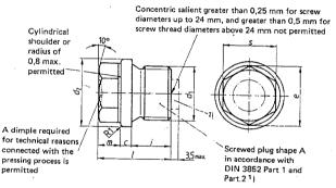
Designation of a steel (St) screw plug with thread  $d_1 = M 20 \times 1.5$ :
