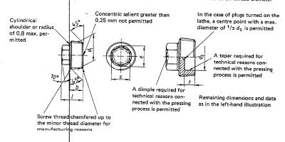
Designation of a steel (St) pide plug with tapered thread  $d_1 = M 20 \times 1.5$ :
