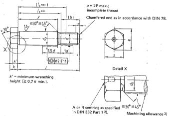
Designation of an M 12 hexagon fit bolt (width across flats: 17 mm), of length l = 60 mm and assigned to property class 8.8 1): Fit bolt DIN 609 - M 12 x 60 - 8 8
