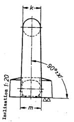
Designation of a lifting eye nut with thread  $d_1$  = M 20: Lifting eye nut M 20 DIN 582
