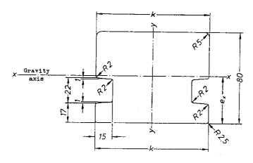
Designation of a crane rail, Type F with head width k = 100 mm: Crane rail F 100 DIN 536
