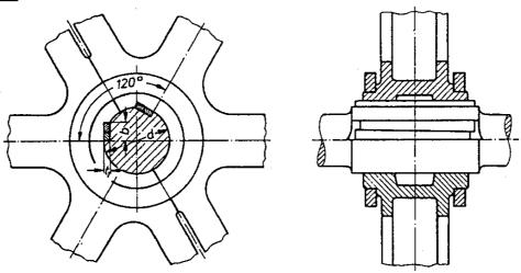
For dimensions d,  $t_1$ ,  $t_2$  and b see pages 1 and 2 The two tangential keys can also be arranged at an angle of 180° should an angle of 120° present assembly difficulties.
