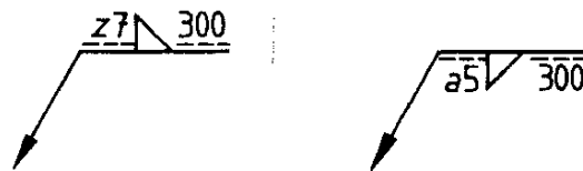
Figure B.2 — Weld on other side
