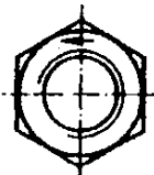
Figure 5 — Left-hand thread marking
